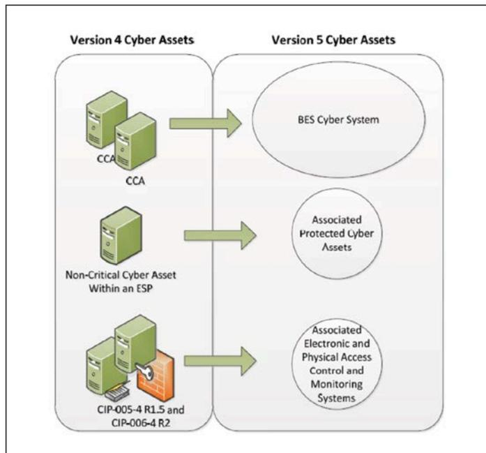
**Figure 1. CIP Version 5 BES Cyber System Categorization**
