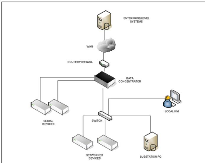
Figure 6. Network Segmentation Using a Data Concentrator
