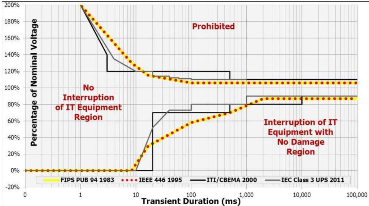
**Figure 6:** Historical perspective of IT equipment disturbance tolerance.
