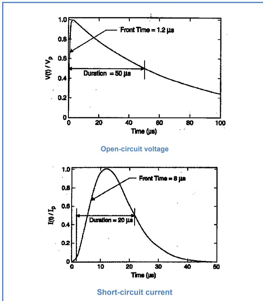
Figure 11: Anatomy of the 1.2 - 8  $\mu$ s combination wave.
