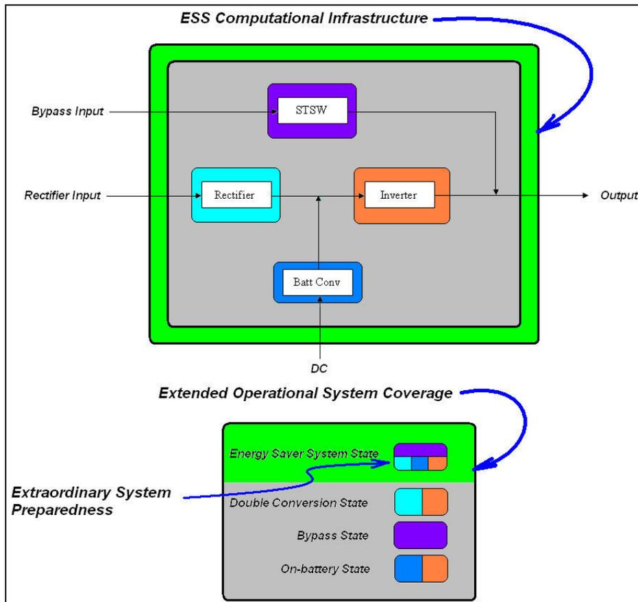
**Figure 4:** Traditional UPS states plus ESS.
