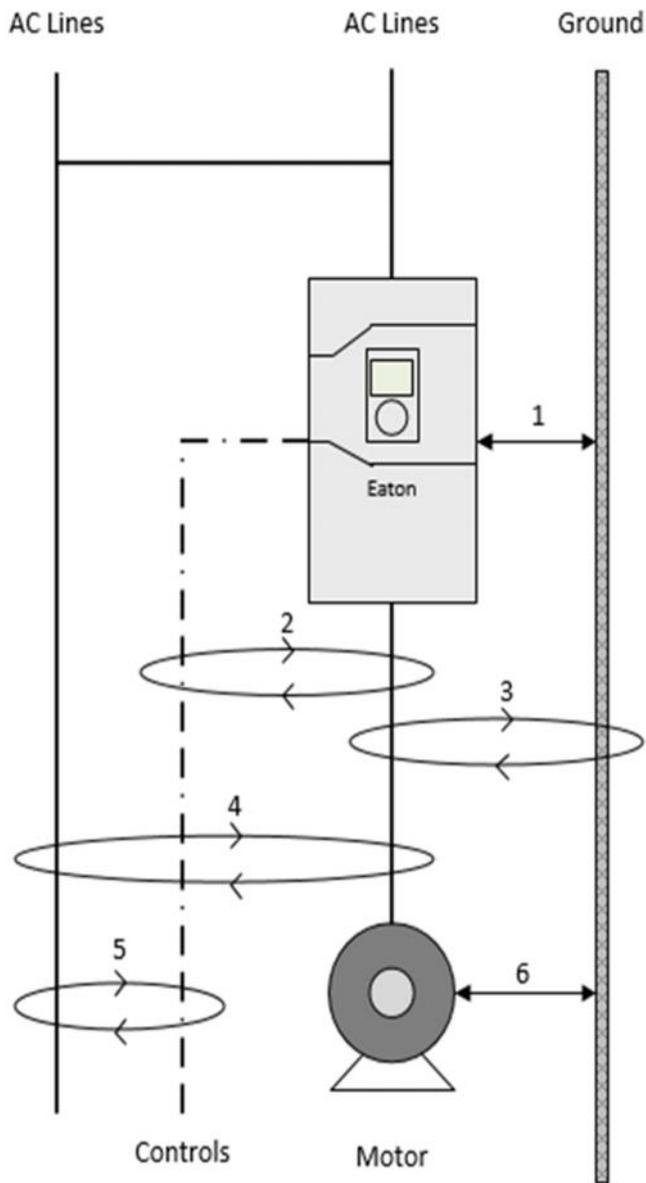
1. Electromagnetic Interference (EMI) can be carried on the ground back to the drive via the ground connection shown above.
